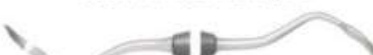
ED-025-315 Crane Kaplan #6 Mirror image blades that taper to a point from a 2.0mm width. The terminal shank is set at 35° to the handle with a reach of 15mm.
