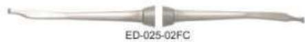
ED-025-02FC Fedi # 2 Tip width = 2.5mm Semi-Circular Cutting Edges on each side and set at a 15oAngle
